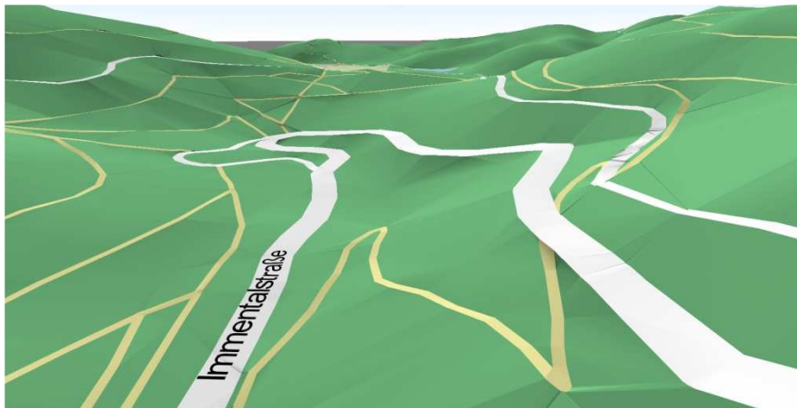
Fig. 12: Some mountain roads integrated into the terrain and flattened. Major roads have a higher priority and have been flattened more than smaller forest tracks.
