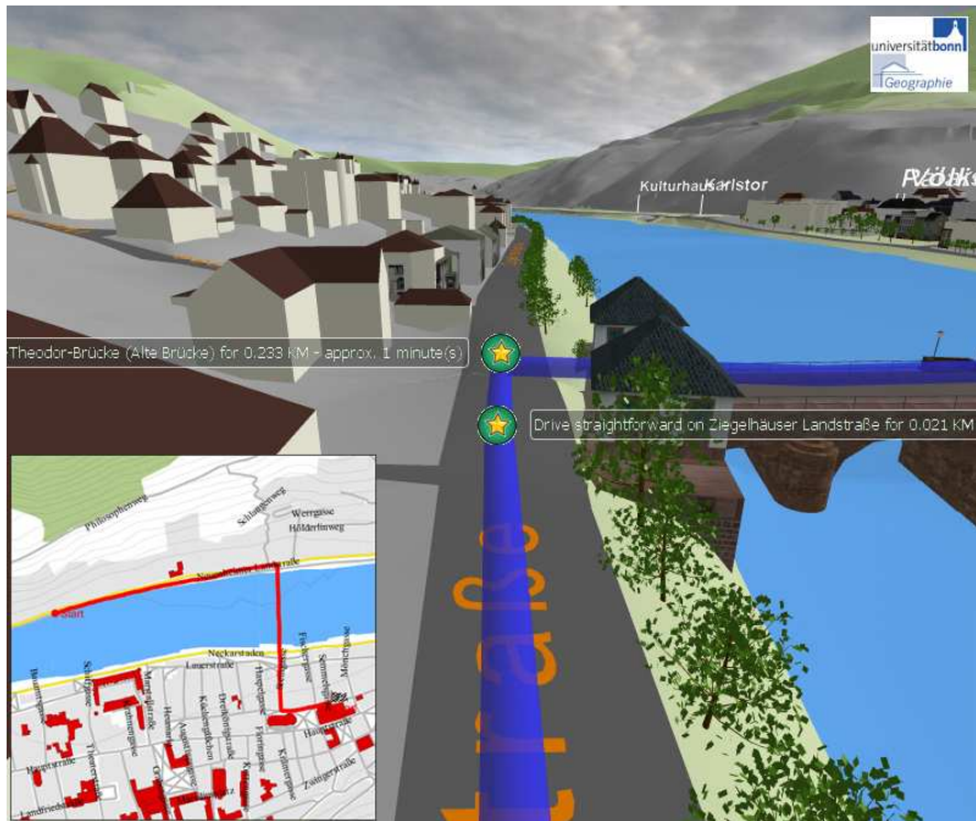
Fig. 9: Display of a route integrated into a 3D city model with corrected road surface. The route goes right onto the bridge.
