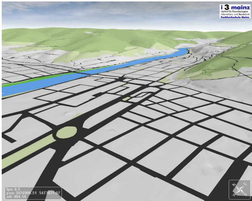
Fig. 9 - Thematic 2D layers integrated into the terrain model
